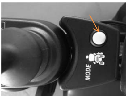
3. Seating Actuator Selection: Push the yellow button on seating selection panel(SSP) to toggle which seating actuator(s) is(are) selected. Move forward/backward the joystick to activate the seating actuator(s)
