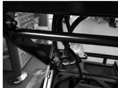
Step 14. Connect the two connectors between rehab seat and seatlift.(if with seatlift.)
