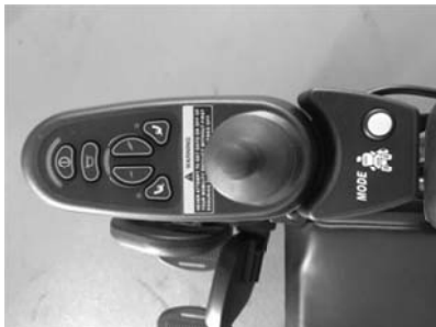
Step 13. Install joystick set
